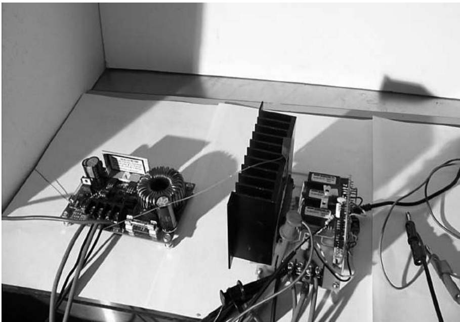
FIGURE 25.7 Power electronics for heater. Left, DC voltage booster; right, IGBT module.
