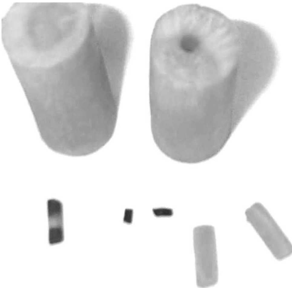
FIGURE 20.1 Picture of alginate spore beads and amylase TTI tubes.
