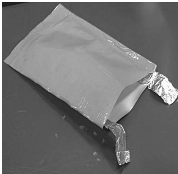
FIGURE 25.1 Original embodiment of Ohmic pouch with protruding electrode tabs.
